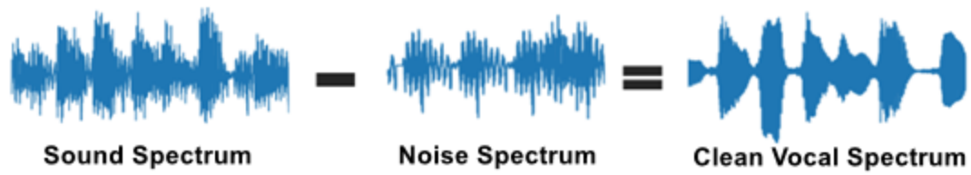
Figure: Conceptual Diagram of Spectral Subtraction
